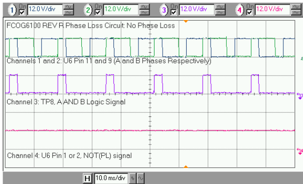
Figure 1. Phase Loss Circuit Signals – No Phase Loss 4 Channels: 1. Digital A Phase Reference Signal, U6 P11 2. Digital B Phase Reference Signal, U6 P9 3. A and B logic signal, TP8 4. \overline{PL} Signal, U6 P1
