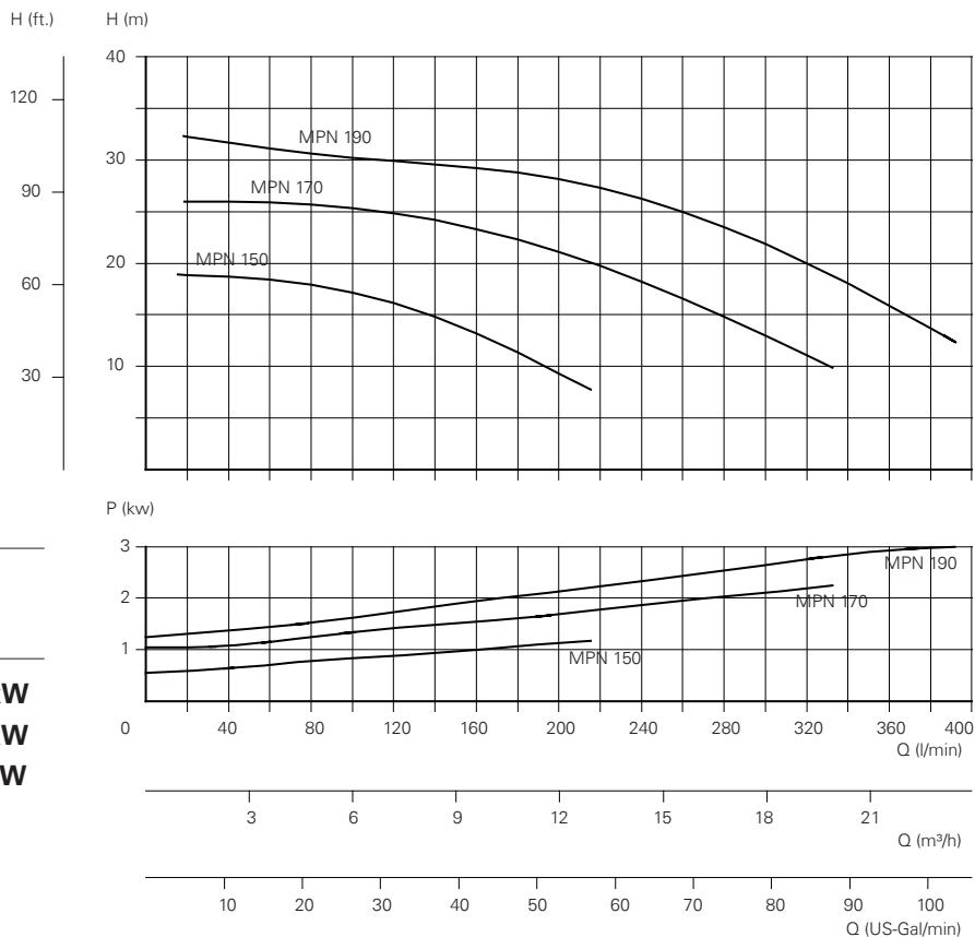
Characteristic lines measured with water, 20° C and 2900 Rpm (50 Hz.)
