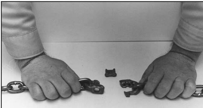
1. Slip the PETOL X86 halves through the chain to be connected.
