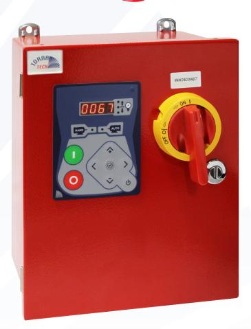
The standard power circuit consists of a horsepower rated disconnect switch, a thermo-magnetic motor protector and a motor contactor for across the line full voltage starting. Consult factory for other types of motor protection or starting methods available.
