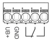
The representation of the relay contact indicates the operating state "Devices connected to voltage supply and no leakage is detected". The relay is energized in this operating state. When condensation or when switching off the operating voltage, it falls off.
