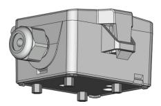
The leakage sensor lies with its own weight on the four contact feet. The detector electrodes are electrically insulated at the lower end, whereby a surface condensation is not detected. The height of the insulation can be variably adjusted, which makes it easy to adapt to local conditions.
