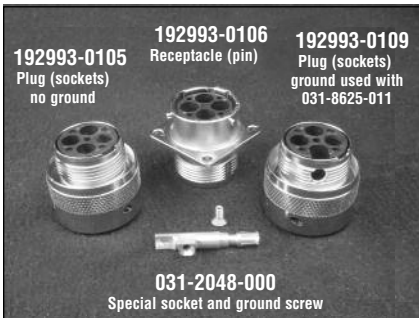
TNM 700 Volt Power Connector System Shell Size 16
