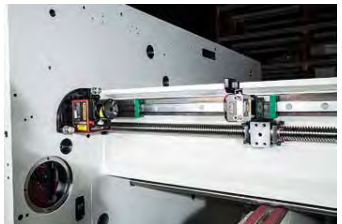
Straightness measurement of linear guide with laser transmitter D22 from system E720.
