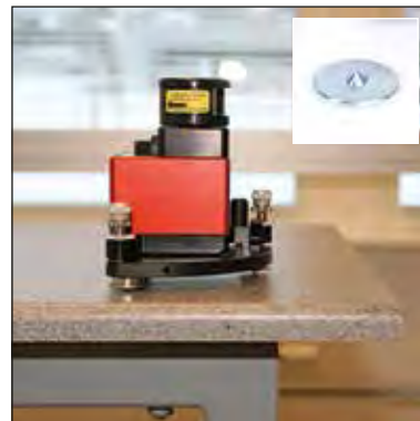
Feet with points (included), on non magnetic surface.
