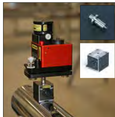
On round surfaces, horizontal sweep. Pin included with D22.
