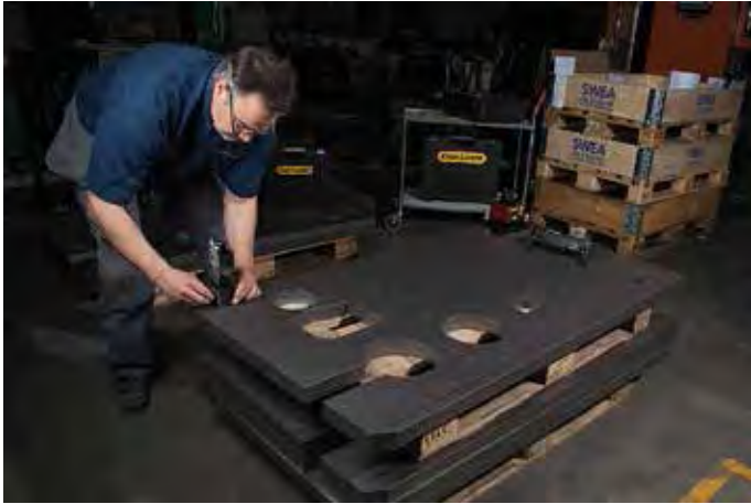
Flatness measurement of machine end after machining.
