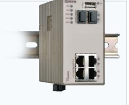
The Lynx 106-F2G is a layer 2 industrial Ethernet switch, powered by the Westermo WeOS network operating system. Lynx is the most compact and has the lowest power requirements in this class of switch. Lynx 106-F2G has 4 10/100 Mbit/s ports in addition to 2 ports which can be fitted with Gbit or 100 Mbit SFP transceivers.
