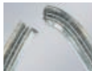
A single-core fiber that is exposed to excessive bending will easily break.
